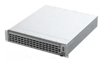
The DS3001 can support port level configuration of sub-rates between 10GbE and 100GbE. System maximum port configuration of 168 10/25GbE, but physically 128 ports of 50GbE (as 2x25GbE) or 64 ports of 100GbE (4x25GbE) using breakout cables provides a superior fabric device for large radix CLOS networks. DS3001 provides superior low latency and power efficiency in a clean PHYless design, while offering high-reliability features such as redundant and hot swappable power supplies and fans.
