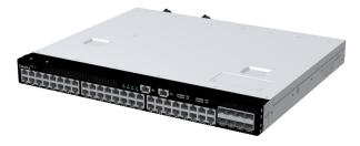
An Open Compute Project (OCP) accepted design, the DS1000 Ethernet switch offers 48 x 10/100/1000Mbps RJ45 ports and 8 SFP+ ports within a 1U form factor. With support for a COM-E modular atom-based control plane, the DS1000 includes an ONIE installer to support third-party network operating systems.
