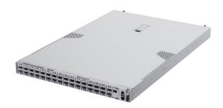
Celestica's DS4000 is a 32 QSFP-DD port 400GbE switch in a compact 1U form factor that provides 12.8Tbps bandwidth for the most demanding data center needs.
